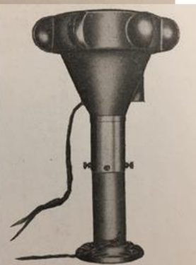
FIG. 28. The rotor-type heated anemometer.
